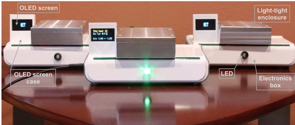
FIG. 1: An array of desktop muon detectors and the corresponding components. When a muon passes through one of the light-tight aluminum boxes, the electronics box records the event and displays the information on the 0.96-inch organic light-emitting diode (OLED) screen. The green light-emitting diode (LED) in the front flashes for a period governed by the number of photons observed by the photodetector. The data can then be transmitted to a computer via a mini-USB cable.
