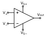
$$V_{out} = A_{OL}(V_+ - V_-)$$
