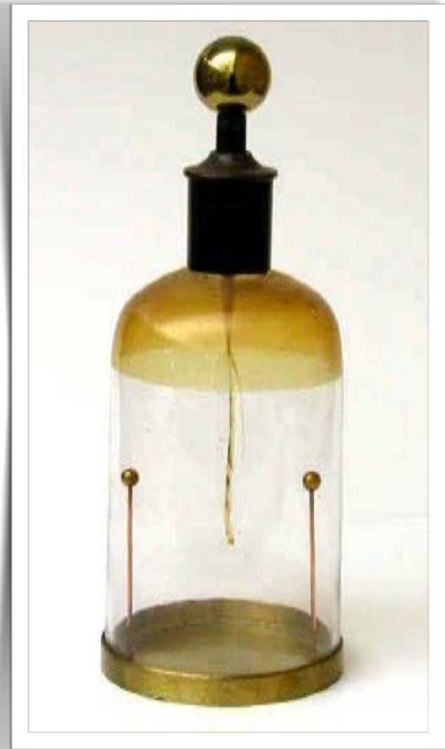
A GOLD-LEAF BENNET-TYPE ELECTROSCOPE (CA. 1880s) MANUFACTURED BY DUCRETET.
