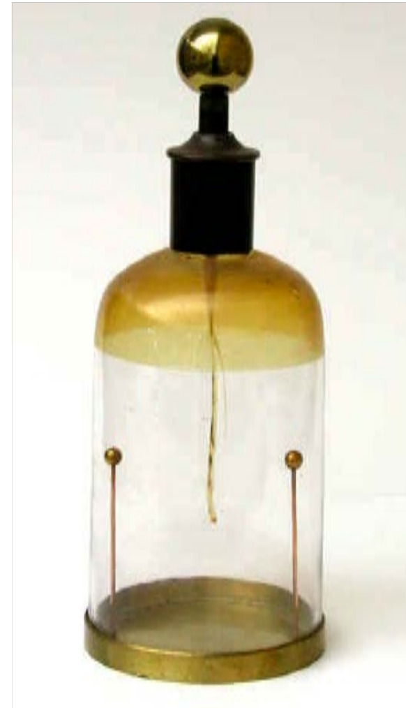
A GOLD-LEAF BENNET-TYPE ELECTROSCOPE (CA. 1880s) MANUFACTURED BY DUCRETET.
