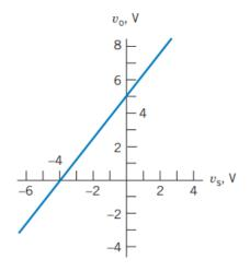
6. Specify values of  $R_3$  and  $v_a$  that cause the output to be related to the input by the equation  $v_o = 4 \cdot v_s + 7$
