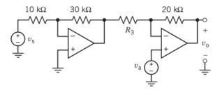
7. Design the circuit so that its input and output have the relationship specified by the graph shown,  $v_o$  is the output and  $v_s$  is the input
