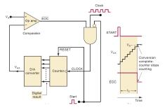
• When conversion process is complete, a  $\overline{EOC}$  is generated and and the contents of the counter are the digital representation of  $V_A$ .
