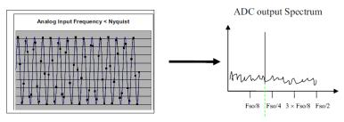
• Examples above refers to a monotone signal, in general the analog input signal bandwidth must be less than the ADC's Nyquist frequency.
