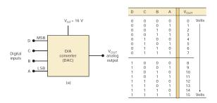
• Notice that there is an input for a **voltage reference**,  $V_{ref}$ . This input is used to determine the **full-scale output** or maximum value that the D/A converter can produce
