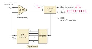
The op-amp comparator has two analog inputs and a digital output that switches states, depending on which analog input is greater
