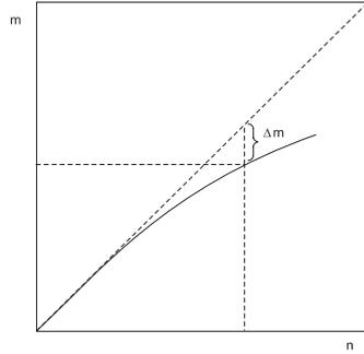
**Figure 12.** The dependence of the rate of counted pulses on the true rate of PMT pulses
