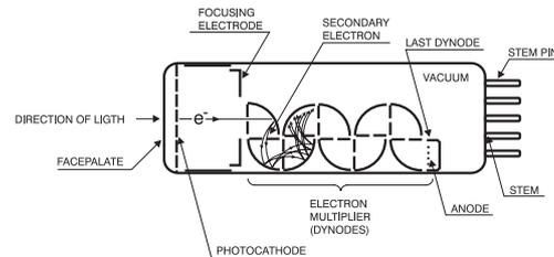
**Figure 1.** Structure of the photomultiplier
