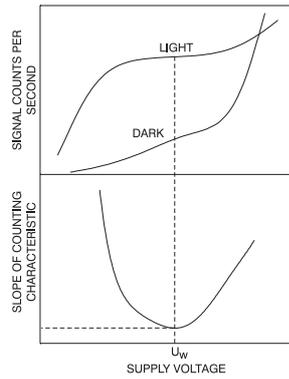
**Figure 11.** The definition of the "working point" of a photon counter
