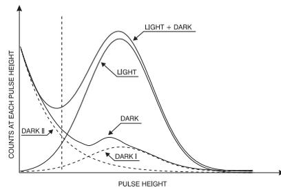
**Figure 6.** PHD of light and dark pulses of PMT output
