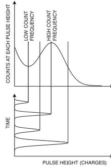
**Figure 3.** PMT output pulses and PHD
