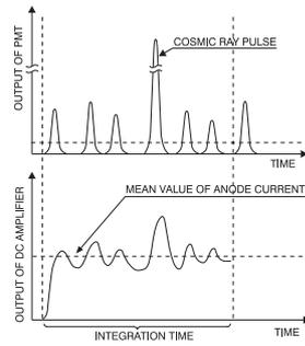
Figure 4. Analogue mode of PMT application
