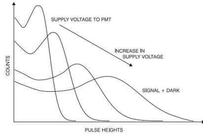
Figure 7. PHD of PMT when the supply voltage is changed
