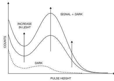
Figure 8. PHD of PMT when the incident light is changed
