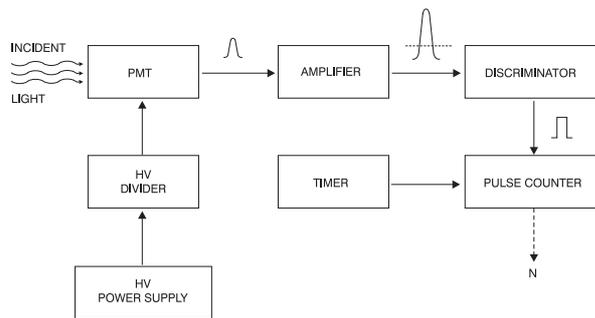
Figure 9. Basic configuration of the photon counting system
