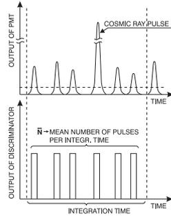
Figure 5. Single photon counting mode of PMT application
