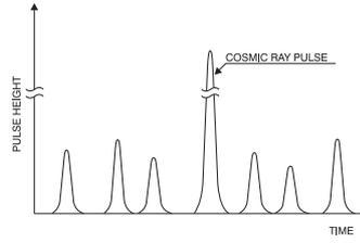
**Figure 2.** Diversity of PMT output pulse heights
